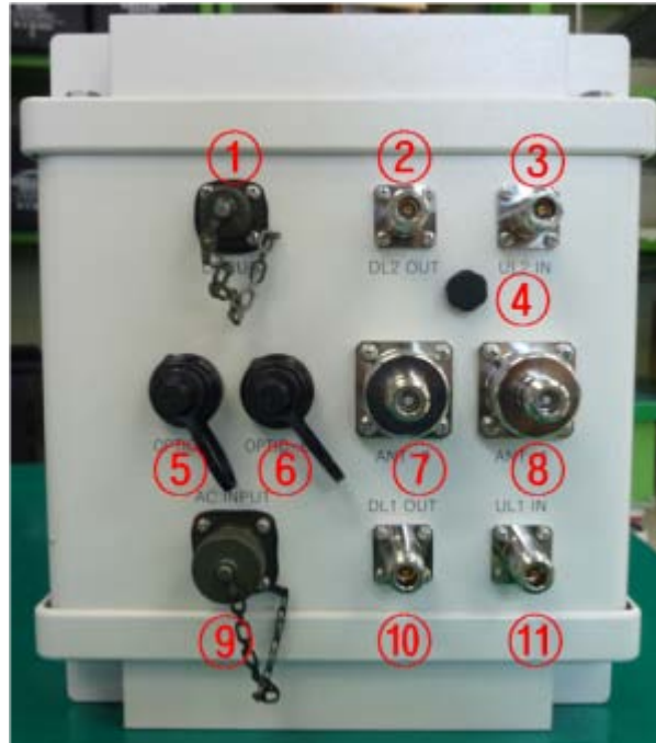
Figure 2-3 Front view of RU system
