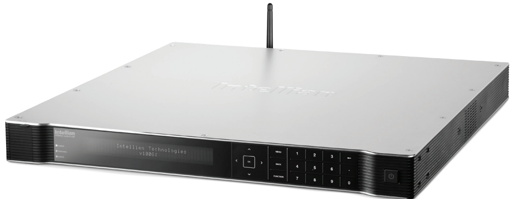
Antenna Control Unit
