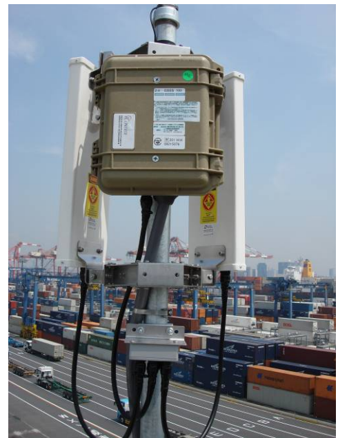
iCHIME Reader utilizing an Internal iCHIME Module
