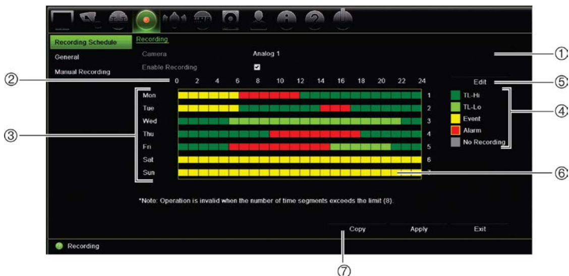
Figure 25: Description of the recording schedule window
