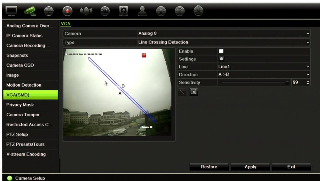
Figure 21: Line crossing detection window
