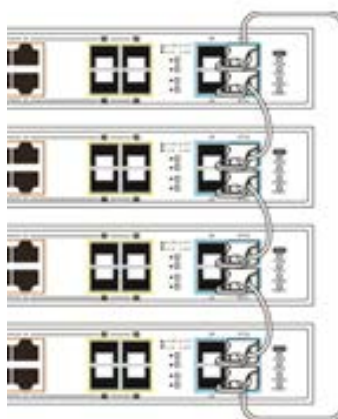
Figure 4-19-2 Ring Stack topology
