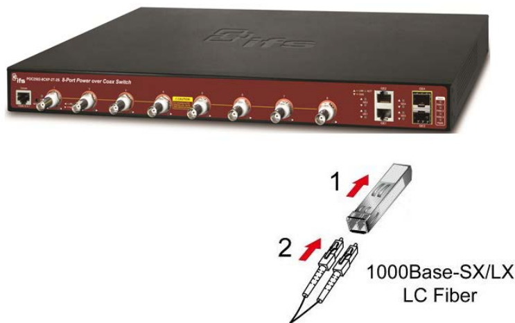
Figure 2-1-7 Plug in the SFP transceiver
