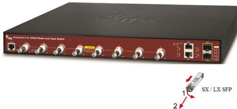
Figure 2-1-8 How to Pull Out the SFP Transceiver
