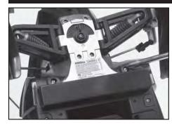
1. Using a Phillips head screwdriver (not included) unscrew the two screws on the battery cover located under the snowmobile near the suspension.
