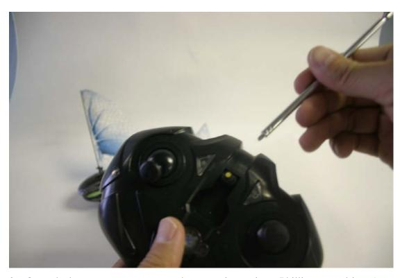
2. Open the battery compartment on the transmitter using a Phillips screwdriver (not included) to remove the screw on the battery compartment door.
