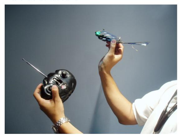
6. On the transmitter, push the right stick (directional) to the left, or push the stick to the right to turn right. The patented technology on VAMP allows the body (alteres) of the insect to roll (left and right) on inputs received from the right control stick. Apply the stick control liberally and turning left and right whilst flying also means it will need space and time to correct its flight path.
