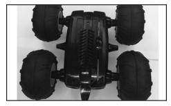
1. Use a Phillips screwdriver to unscrew the battery compartment door. Remove the battery from the Squeeler. Note: Always remove the battery from the Squeeler during charging as this keeps the battery cooler. Never leave the battery unattended while charging.
