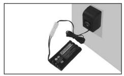
3. Plug the charger adaptor into the AC wall outlet. A typical charger takes 4 hours to complete. After charging unplug the battery from the charger and unplug the charger from the wall.
