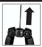
2) Fully extend the antenna on the transmitter and ensure that the transmitter is turned on.
