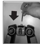
1) Insert the antenna into location on the top of the transmitter and tighten.
