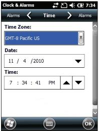
Use the Tile bar to navigate between screens and within applications. The icons available on the Tile bar change depending on the application you are using.
