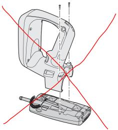
chg or del IP30 does not require screws for attachment
