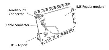
The IM5 Reader Module has holes along the sides that can be used for mounting. For best results, attach heat sink to case via the screwholes in the heat sink.
