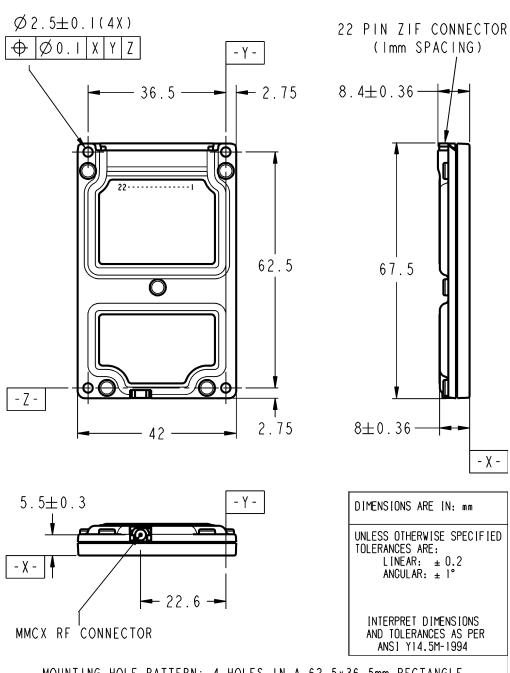
MOUNTING HOLE PATTERN: 4 HOLES IN A 62.5x36.5mm RECTANGLE.
