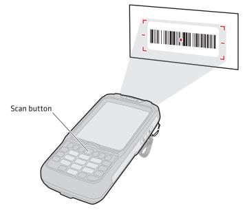
**4** Use the laser pointer as a guide and aim toward the middle of the bar code. Make sure that the illumination frame covers the bar code you are trying to decode.
