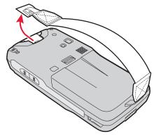
**4** Push forward on the battery release tab until the battery releases, and then lift it away from the CN50.
