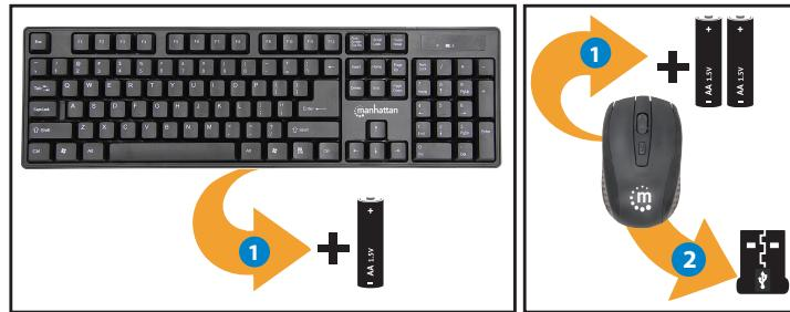
**1** Insert the supplied batteries into the wireless keyboard (1x AA) and the wireless mouse (2x AAA).
