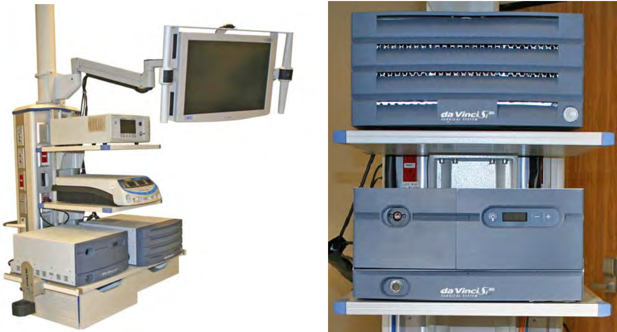
Figure D.1 Recommended side by side (left) and stacked (right) VisionBoom configurations
