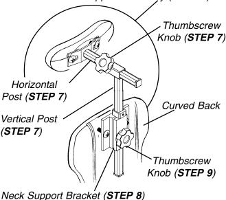
NOTE: Ensure that the retaining screw is located in the end of the horizontal post.
