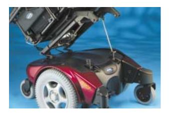
The PTO Plus integrates into the base of the chairs while still maintaining easy battery access through a simple flip back design
