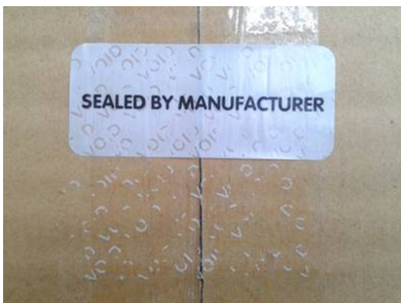
Fig. 2.2: Bad tamper seal
