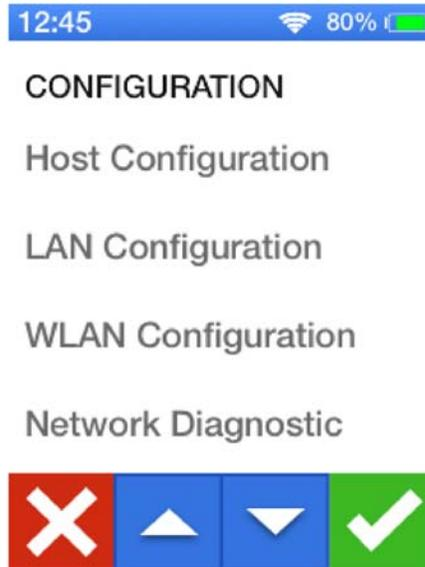
Located on the bottom of the Main Configuration Screen is the Configuration Navigation Bar. In this Configuration Navigation Bar, it contains buttons that will (1) Cancel, (2) Up and Down Buttons and (3) Confirm the actions made during the time of entering the Main Configuration Screen.
