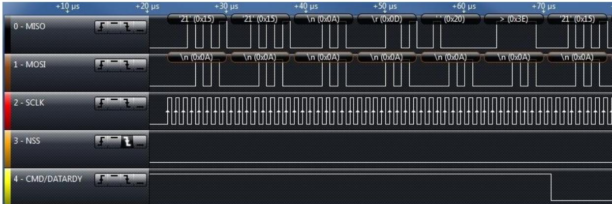
The endian requirement extends to the command being sent to the **eS-WiFi** module. So a “I?\x0A” command would be sent as 0x3F 0x49 0x0A 0x0D.
