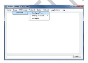
You will now configure the VSP (Virtual Serial Port) connection the EVB. You will need to determine what COM port is attached to the EVB. This can be done by using Windows Device Manager. In this case, COM54 is the port connected to the EVB.
