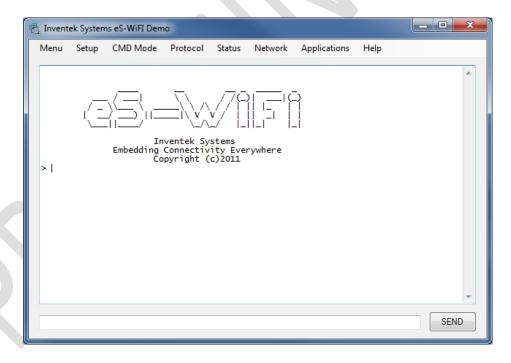
The eS-WiFi module is shipped with the default serial configuration of 115200 baud, 8 data bits, no party, and 1 stop bits.
