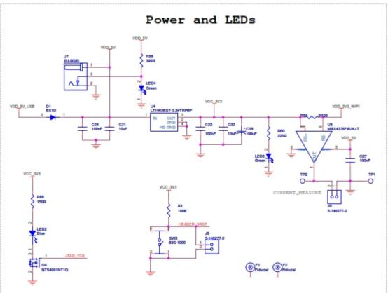
Errata: Current measurements are not supported with the EVB. U5 pins 4 and 5 are reversed on the PCB. So you cannot take current measurements as delivered. Inventek will fix this on our future EVB builds.
