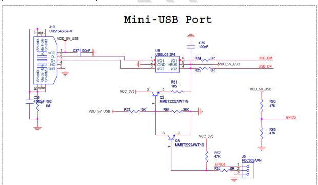
Note: Second USB port J10 is not installed. This is a direct USB connection to the es-WiFi module. This evaluation board is for UART only. Contact Inventek is you are interested in USB
