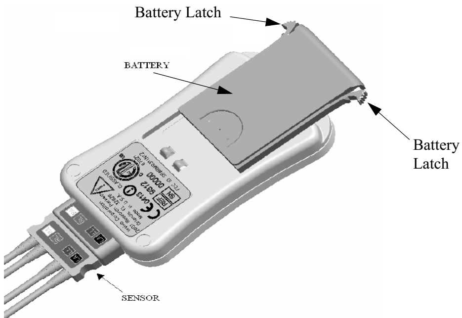
Figure 2-4. WECG Module Battery Location
