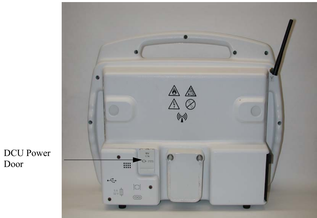
Figure 2-11. DCU Power Input
