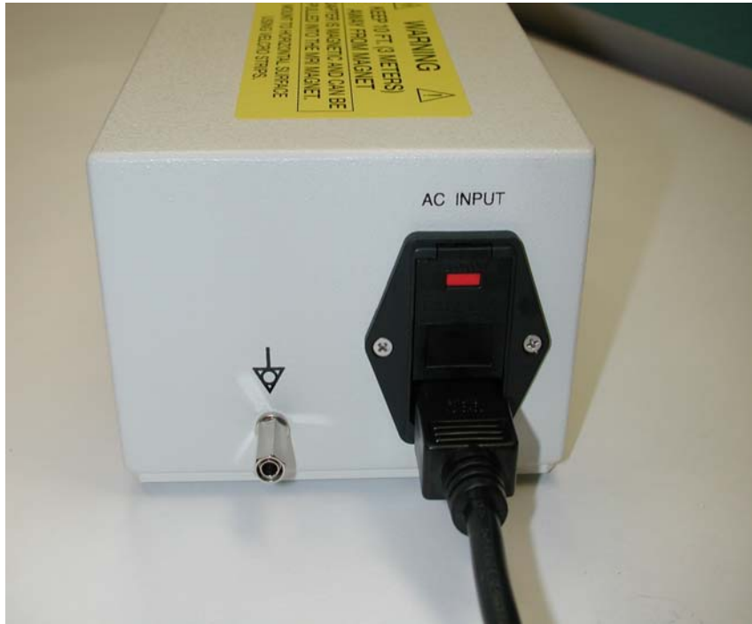
Figure 2-8. AC Power Connection To Precess AC to DC Power Supply (Part Number AS201)
