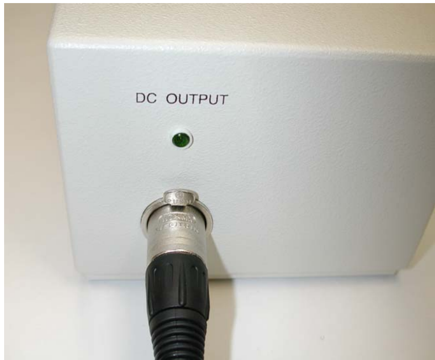
Figure 2-9. Precess DC Power Connection To Precess AC To DC Power Supply (Part Number AS201)
