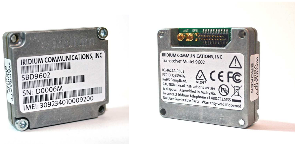
Figure 1 Iridium 9602 SBD Transceiver Front and Back Views
