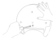
Figure 5: Screw in 1 1/2 screws into plastic wall inserts
