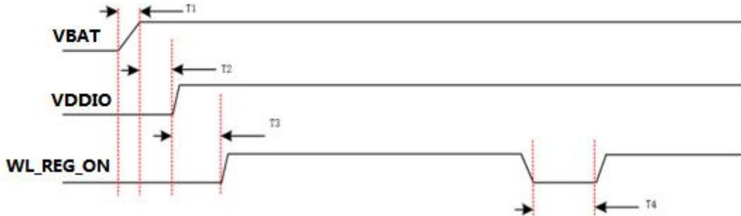
Figure 4. Power-up and Power-down Timing of SW6621-44B1
