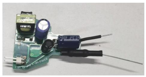
2.2. Locate an available slot and carefully insert the adapter. Solder the adapter to the motherboard using a tin wire
