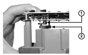
**9.** Install and tighten the left-hand index mounting screw (for indexes with either mounting screw slots or holes). Use one 8 - 32 x 3/16-inch screw for this step (you can use an original mounting screw if it was the correct size and not corroded; otherwise, use the correct size replacement screw).
