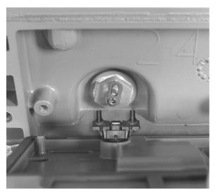
**3.** Gently place the ERT module assembly on the meter. Align the four screw holes on the ERT module assembly with the holes on the meter.
