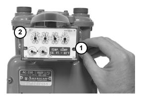
**6.** Press the new tamper seals into place using the 11/32-inch nut driver (or another similar blunt tool).
