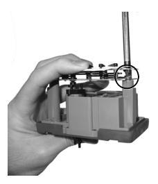
**6.** If the index has mounting screw *slots*, screw an index mounting screw (1) one to two turns into the ERT backplate's right-hand index mounting post (2). Use one 8 - 32 x 3/16-inch screw for this step (you can use an original mounting screw if it was the correct size and not corroded; otherwise, use the correct size replacement screw).
