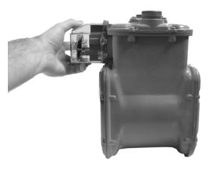
**4.** Turn each screw 1/4 to 1/2 turn after it contacts the cover. Use the 1/4 - 20 x 5/8-inch screws for this step. You can use the original mounting screws if they were the correct size and not corroded, otherwise, use the correct size Replacement Screws on page 14.
