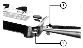
**5.** Attach the screw to the ERT backplate's right-hand index mounting post just far enough to hold the screw and end of the index in place.
