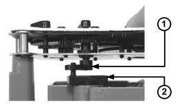
• If the index wriggler has a drive post (1), place the index wriggler's drive post in the backplate wriggler's drive slot (2).
