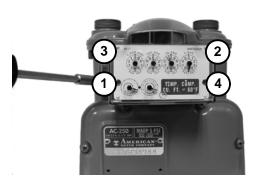
**5.** Place a new tamper seal over two of the mounting screws as shown below.
