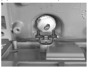
• For Two-Foot Meters: Align the ERT module assembly wriggler with the meter drive slot (as shown below). It is acceptable for the pin on the 100G wriggler to be installed inside or outside of the meter drive slot. For ease of assembly, Itron recommends that the pin on the 100G wriggler be installed outside of the meter drive slot.
