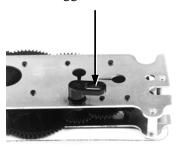
• Index wrigglers on two-foot meters have drive posts.
