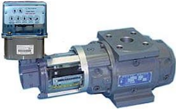
100G DLS Elster American commercial gas ERT module mounted on a GE Dresser Meter with an instrument drive
