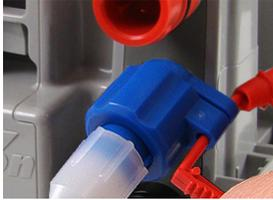
2. Insert the pointed end of the security seal into the capped end and push until the seal locks.
