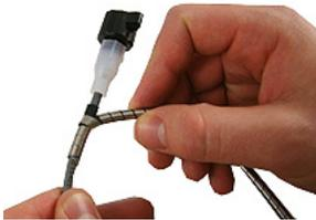
**Warning** You must begin wrapping the cable armor over portion of the cable protected by the electrical tape. If you do not begin to wrap the cable armor over the protected portion of the ERT module cable, a cut cable could cause an ERT module/register communication failure.
