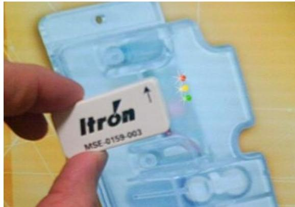
2. Watch the red LED blink pattern to verify that the range extender is searching for the configuration devices.
