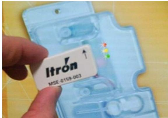
The range extender searches for CENTRON meters and attempts to join the meter with the best signal quality.
