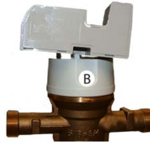
B. Incorrectly mounted 80W-i
