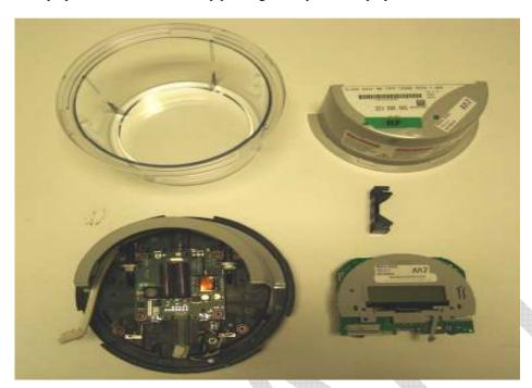
Connect metrology and the ACT2 module using the board to board connector.
