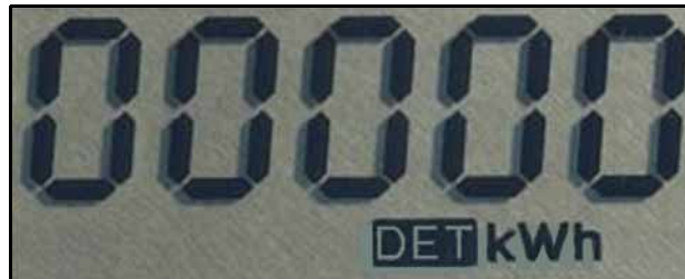
Figure 4.10 Delivered kWh with Detent Enabled
