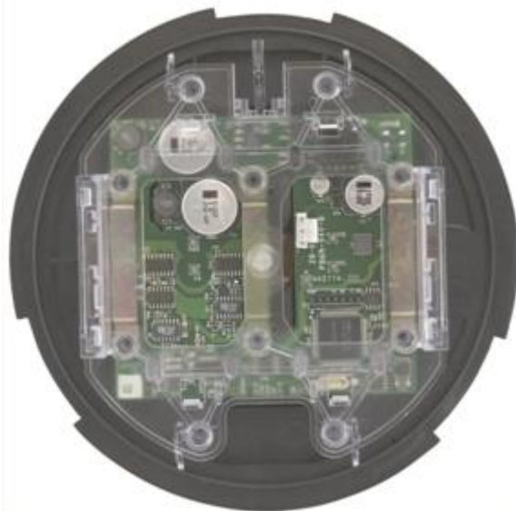
Figure 1: CENTRON Polyphase Meter Metrology
