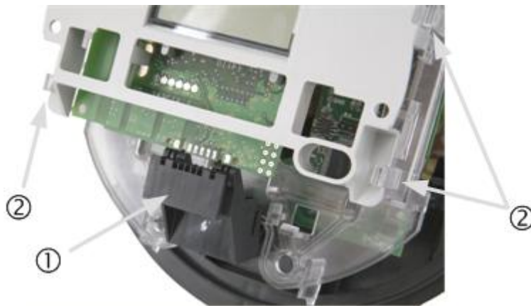
Figure 4: Removing the Board-to-Board Connector
