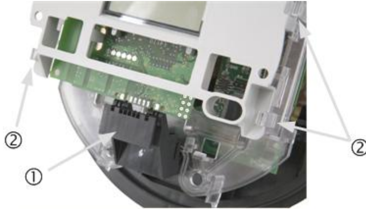
Figure 4: Removing the Board-to-Board Connector
