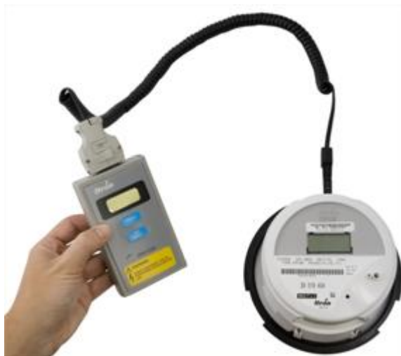
Figure 12: ZRO-C2A Resetter Connected to the CENTRON
