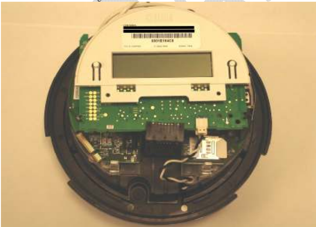
Meter Base with CAT1 and register boards installed
