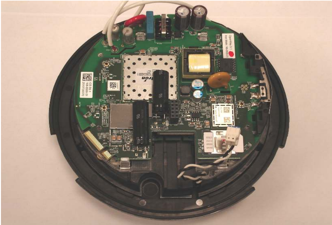
Meter Base with CAT3 and register boards installed
