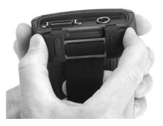
Place the FC200 face down on a clean surface and insert the battery into the battery compartment. Press the top edge of the battery pack firmly to ensure that the power connector engages securely.
