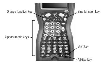
The **Orange** and **Blue** function (FN) keys are located at the upperleft and upper-right corners of the keypad. These provide access to the orange and blue characters and functions printed above each alphanumeric and cursor key.
