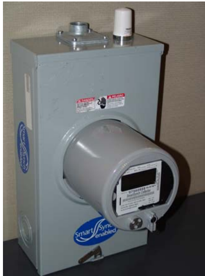
FIGURE 1 Mounting example of Laird/Antenex antenna directly to meter panel.
