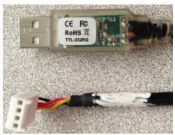
Figure 1: Serial-To-USB Adapter cable
