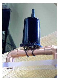
The MLOG logger is attached directly to the pipe using one (1) buna O-ring, as shown to the left or one cable tie, as shown on the right.
