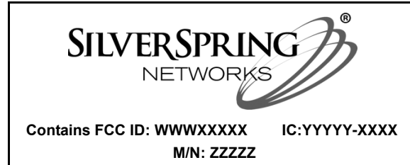
Figure 8. Sample FCC ID label for devices containing a NIC
