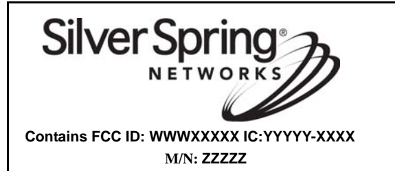
Figure 8. Sample FCC ID label for devices containing a NIC
