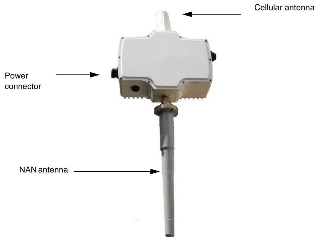
Figure 2. Silver Spring Networks Access Point (AP)
