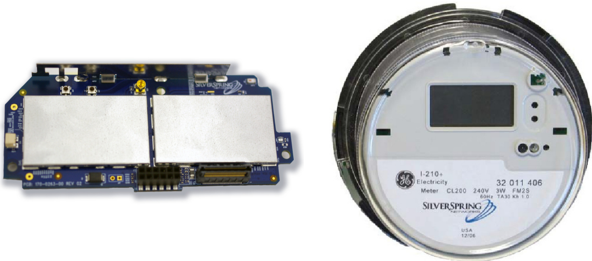
Figure 1. I-210+ NIC and meter
