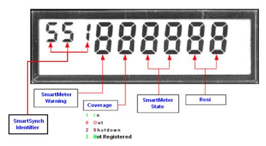
Note: These display codes are only visible when the SmartSynch Option Board type is selected in the meter program and the option board fields are enabled.
