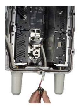
6. Route the PLC signal cable through access hole and secure the cable gland into the threaded hole. Use a 15/16" combination wrench to secure the gland.
