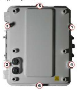
7. Affix the regulatory label (included in the CAM installation kit) to the bottom of the CGR in the label location provided between the antennas.
