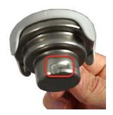
5. Turn the Riva Leak Sensor to lock the sensor into place.
