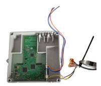
6. Place the cable connection into the remote water module housing with the cable ties to the inside.
